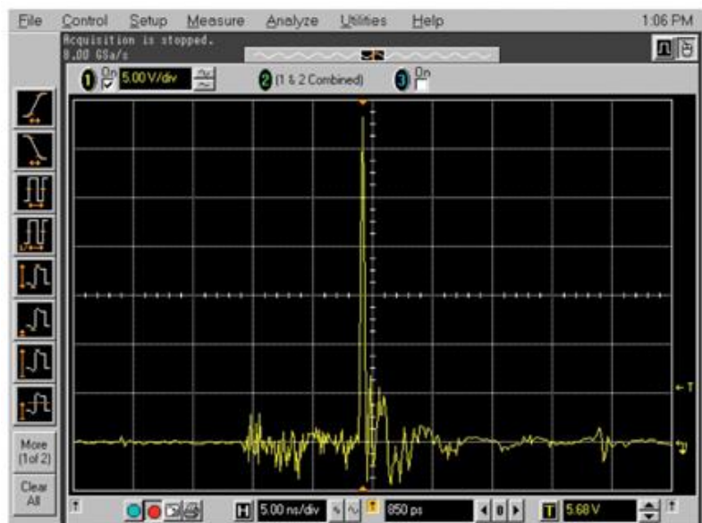
Figure 2: Example of ESD Induced Error in a Digital Oscilloscope
